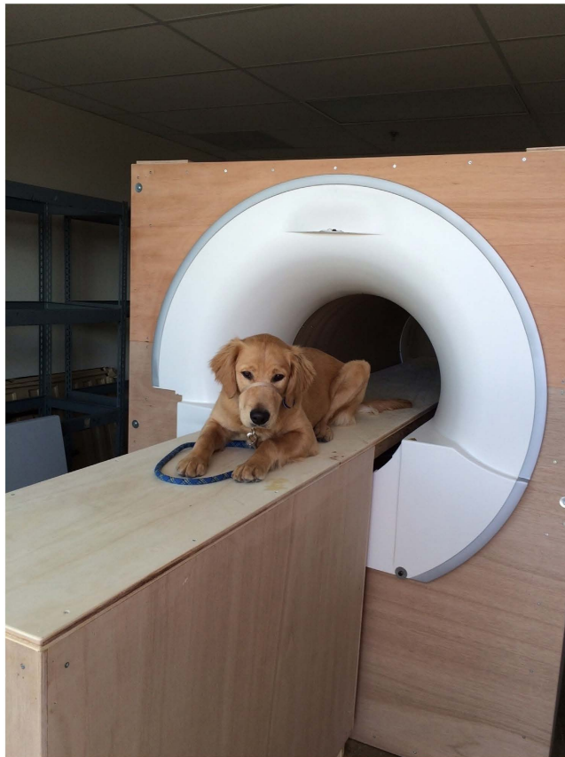
Figure 1. Mock scanner. A dog is shown on the patient table. Speakers to simulate the acoustic noise are inside the simulator.
